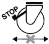
Overload through movement while stopped
